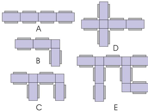
Fig. 4. Several possible minifactory configurations realizable with rectangular and square platen tiles. Each rectangular tile is supported by a base unit.
