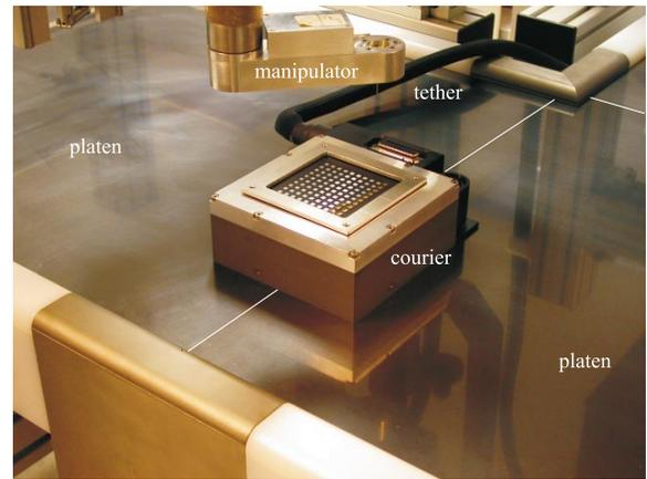
Fig. 6. Courier operating over the interface crack between two tiles (crack emphasized for clarity).
