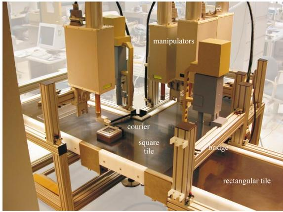
Fig. 2. Photograph of a section of our laboratory minifactory (under development).
