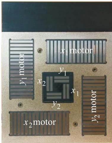
Fig. 5. Courier agent: Bottom view of courier showing motor sections and 3-DOF ac-magnetic position/orientation sensor.
