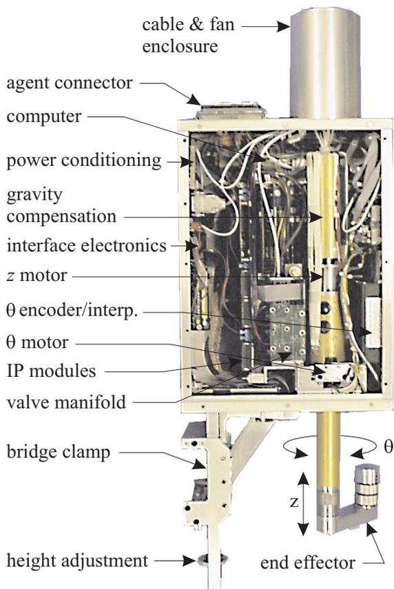
Fig. 7. Two-degree-of-freedom ( $z - \theta$ ) manipulator agent (cover removed)
