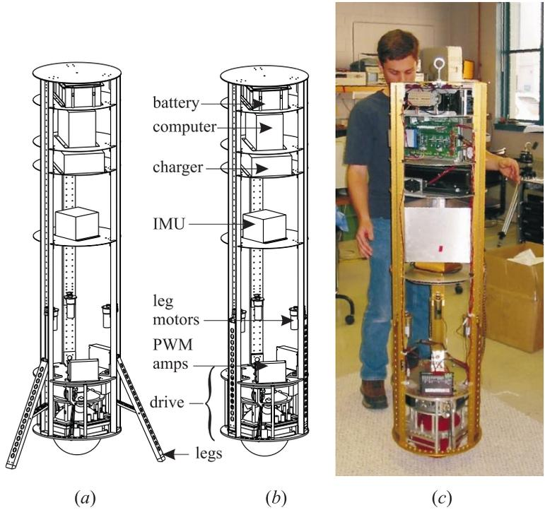
Figure 1: Ballbot design and realization: (a) with three legs deployed, (b) with legs retracted into body, (c) balancing and station keeping.
