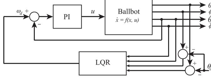
Figure 4: Structure of stabilizing linear feedback controller.
