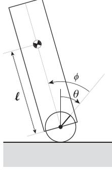
Figure 3: Planar simplified Ballbot model used for controller design.
