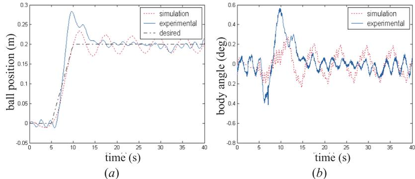
Figure 5: Moving between two locations in a straight line: (a) ball position in meters, (b) body angle in degrees.
