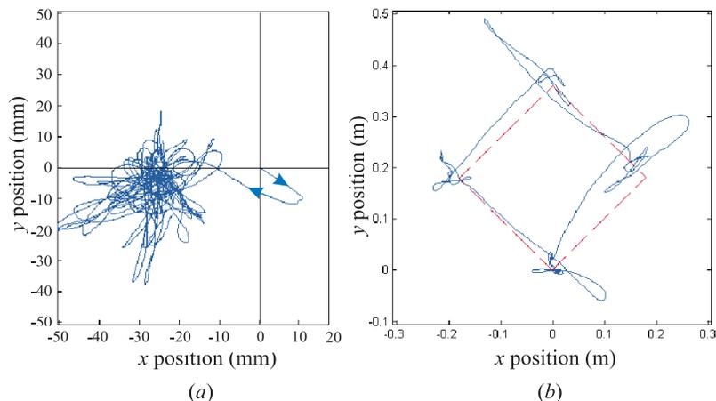
Figure 6: Plots of the ball path during (a) balancing and station keeping, and (b) attempting to move in a square.
