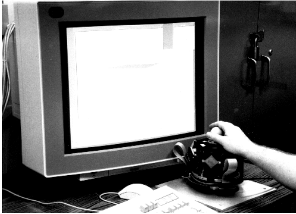
Figure 2: Using the Magnetic Levitation Haptic Interface with a Graphical Display
