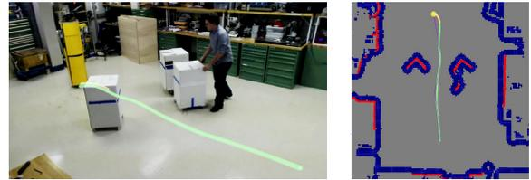
(a) The ballbot initially starting at rest at  $t_0 = 0$  s. A straight path to the goal in the lower right is planned.
