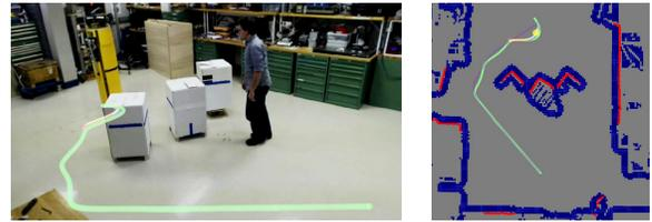
(c) At  $t_1 = 4$  s, a box is placed blocking the straight line path, and the ballbot replans smoothly to go around the obstacles.
