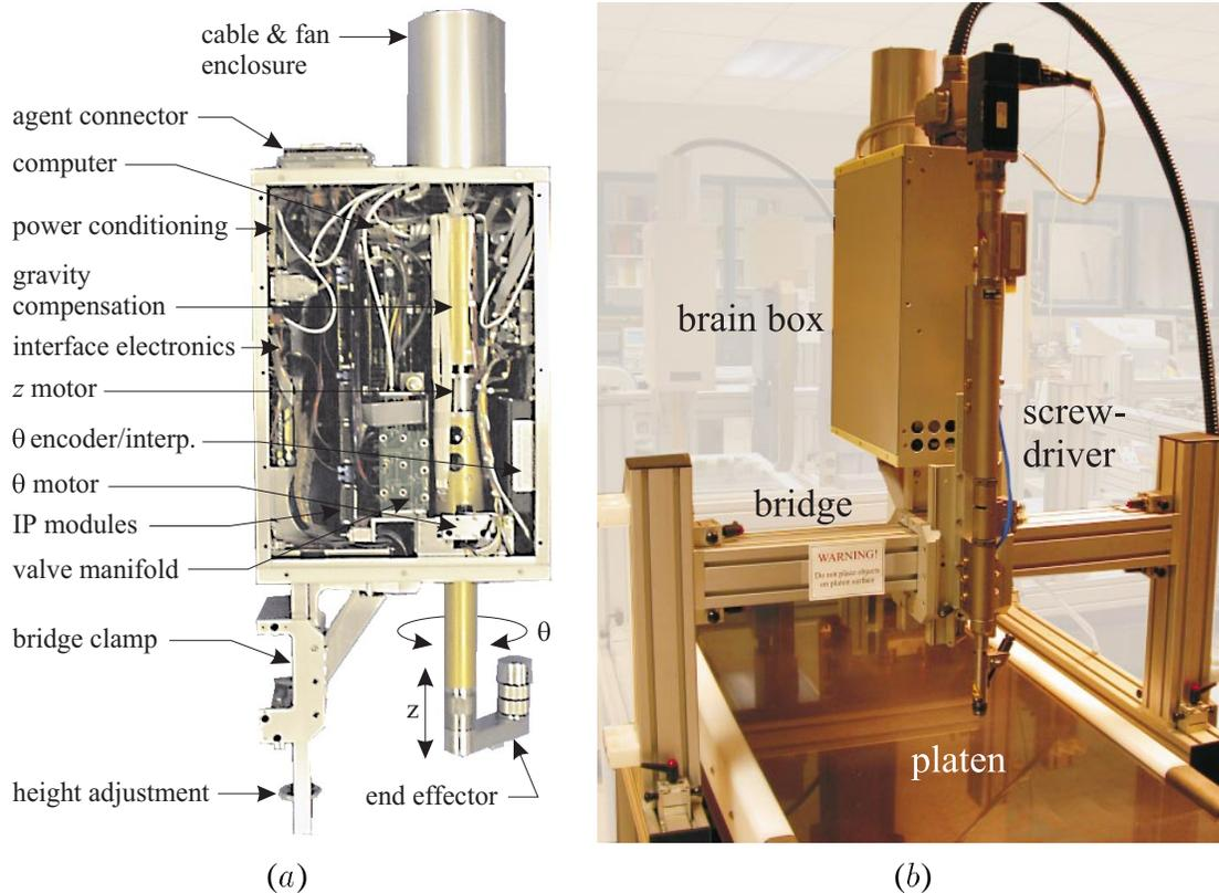
Figure 5: (a) Two-degree-of-freedom ( $z - \theta$ ) manipulator agent (cover removed), (b) Weber Screw-driving Systems automatic screwdriver agent (under development).
