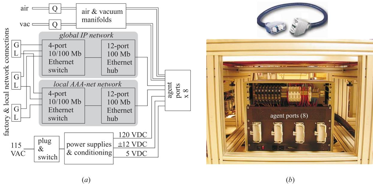
Figure 2: Minifactory base unit: (a) block diagram, (b) photograph.
