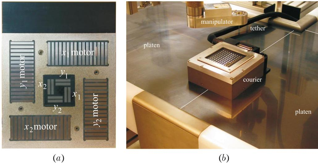
Figure 4: Courier agent: (a) bottom of courier, (b) courier operating over the interface crack between two tiles (crack emphasized for clarity).
