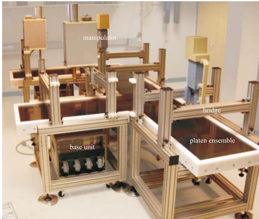
Figure 1: Overall view of minifactory (under construction).
