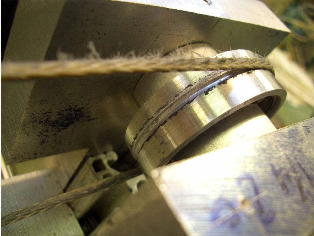
Figure 5.13: After just a few seconds, the cable started to fray, and leave a waxy substance on the pulley. We speculate that high internal damping leads to sufficiently high temperatures to melt the cable.
