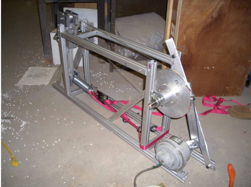
Figure 5.12: The test setup for Vectran cable. A DC motor on the bottom right runs a linkage, which rotates the large pulley at the upper right of the device back and forth. The cable then rolls back and forth repeatedly on the small pulley at the upper left.
