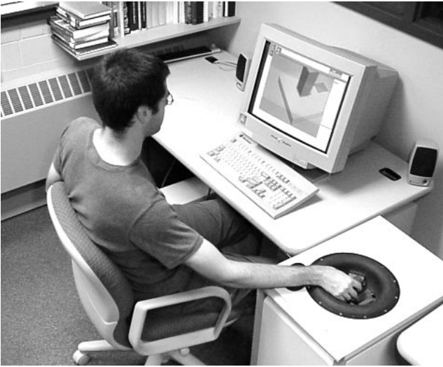
Figure 6: Subject using haptic device during peg-in-hole task.
