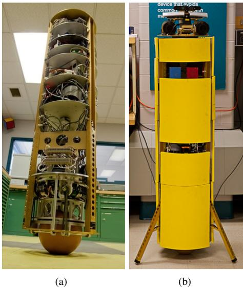
Fig. 2. The ballbot: (a) balancing on its single spherical wheel; (b) with protective skin, blue and red blocks on object deck, and in a statically stable charging configuration (legs down).
