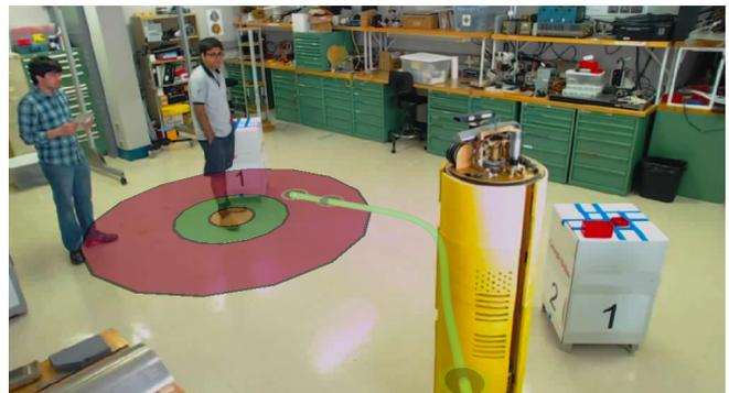
Fig. 5. The curved trajectories planned and executed by the ballbot respect intimate and personal zones of the subject, whereas the straight line paths do not necessarily do so. Proximal zones are shown around subject: Intimate - Orange, Personal - Green, Social - Red
