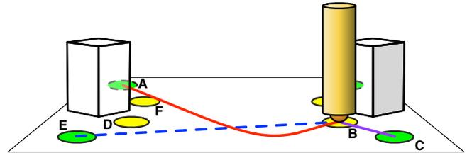
Fig. 4. Experimental Setup - Shown in red is a curved path, in blue a straight path. Yellow ellipses are the goals that either the robot or subject would go to. Green ellipses show the staging areas that the ballbot would move to between approaches.
