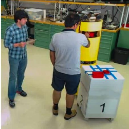
Fig. 1. Subject exchanging objects (red) from the white task location to the robot (yellow). Participants exchanged these “sensors” after each approach. The experimenter is to the left observing the interaction.
