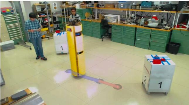
Fig. 3. Trajectories were planned and sent to the controller with a maximum execution length of 2.5 s (shown in blue). If the controller did not receive another trajectory, it would revert to a planned backup stopping trajectory (shown in red). Note that these trajectories are superimposed on the real scene in real time by an augmented reality technique similar to that of the first down line display in NFL football. The operator could see this display during the experiment.
