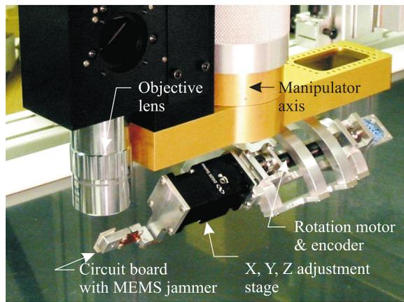
Fig. 8. Minifactory 5th axis mechanism for 3D MEMS assembly.
