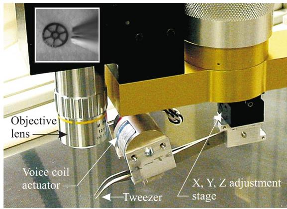
Fig. 5. Minifactory end effector with voice-coil actuated tweezers. Inset: 500  $\mu\text{m}$  LIGA gear and tweezers tips.
