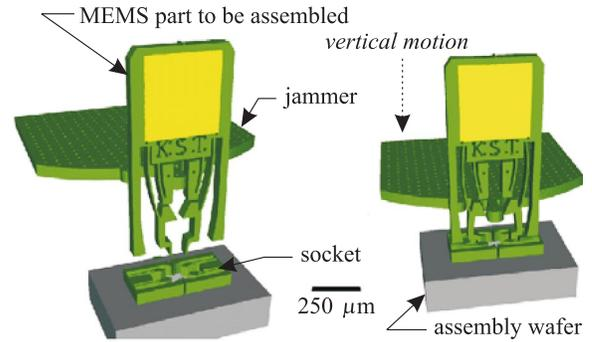
Fig. 6. MEMS jammer and socket configuration during assembly.
