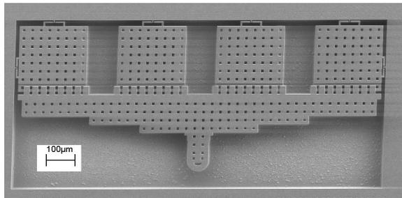
Fig. 9. CMOS-MEMS jammer with integrated piezoresistive force sensing.
