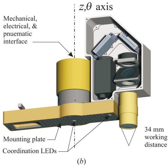
Fig. 2. CAD model of developed microscope end effectors: (a) upper view showing internal parts, (b) lower view showing electromechanical interface, mounting plate, and coordination LEDs.
