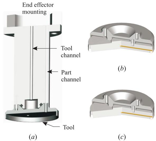
Fig. 3. Vacuum/pressure pick and place: (a) effector design, (b) tool and lens, (c) tool and ring.
