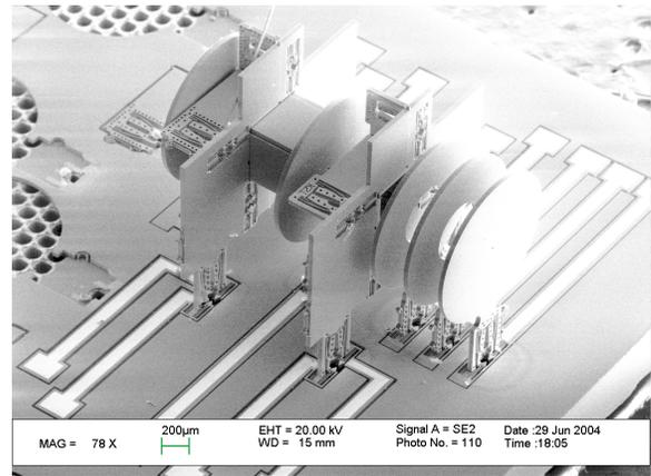
Fig. 7. 3D MEMS assembly produced in the ZyveX Membler system.
