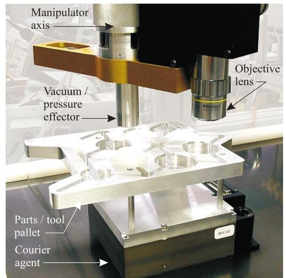
Fig. 4. Parts for an optical assembly, along with associated tools, are carried on a pallet by a courier agent.
