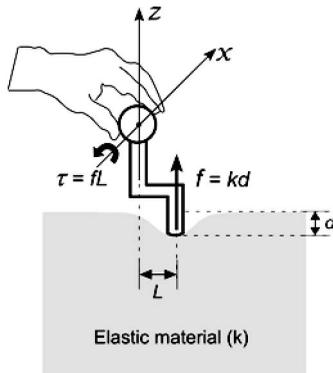
Fig. 1. Force and torque feedback produced by the tool interacting with soft tissue. Rotation is centered in the handle and about the  $x$ -axis.  $L$ ,  $d$ ,  $k$ ,  $f$ , and  $\tau$  denote moment arm length, amount of deformation, stiffness, resisting force, and torque, respectively.
