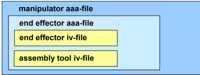
*Figure 11: Nesting levels of manipulator files*
