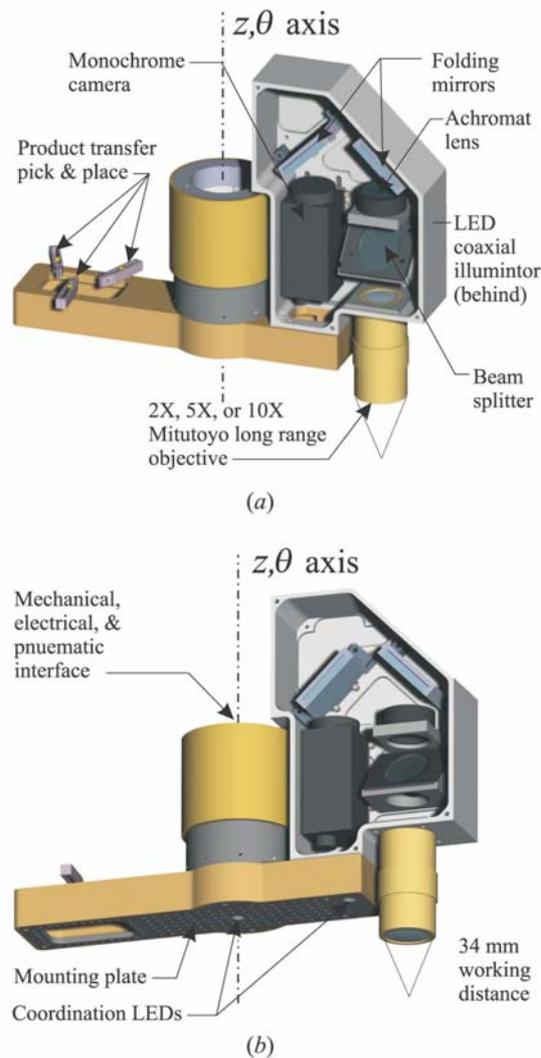
Figure 12: New end effector with attached camera
