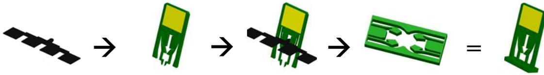
*Figure 24: Assembly principle of the micro mirror*
