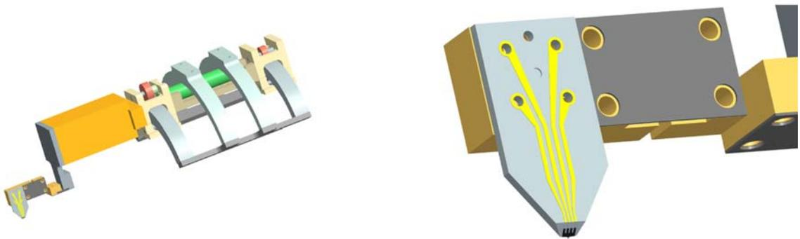
*Figure 25: ZYVEX effector mechanism with attached jammer*
