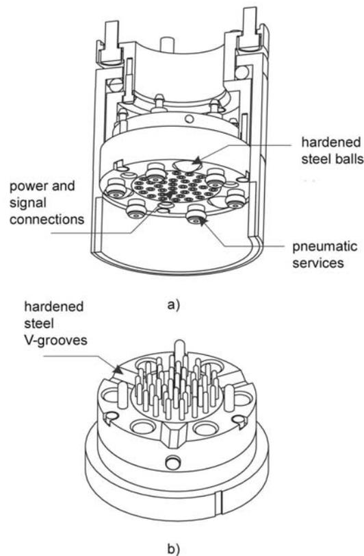
*Figure 3: Connecting interface between manipulator and end effector: a) female connector, b) male connector*
