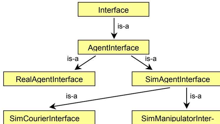
Figure 7: Class diagram for agents Interfaces
