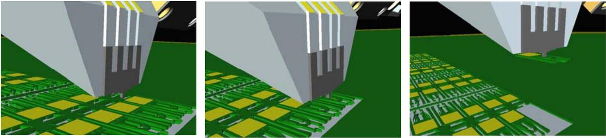
Figure 31: *Detach and pick up of a micro mirror*
