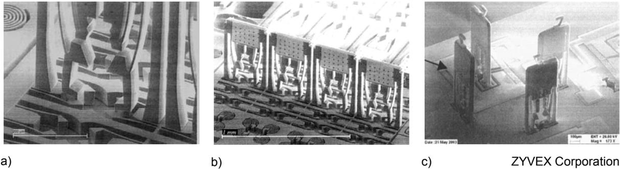
*Figure 20: a) Magnification of the connection, b)+c) 3D MEMS structures*
