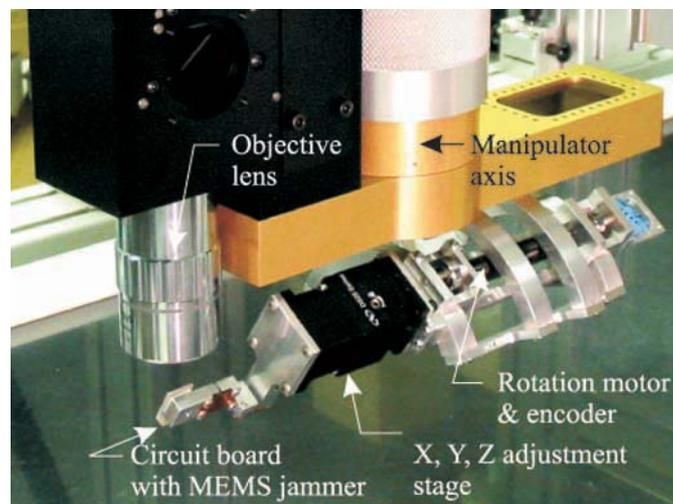
*Figure 27: New end effector with attached effector mechanism*
