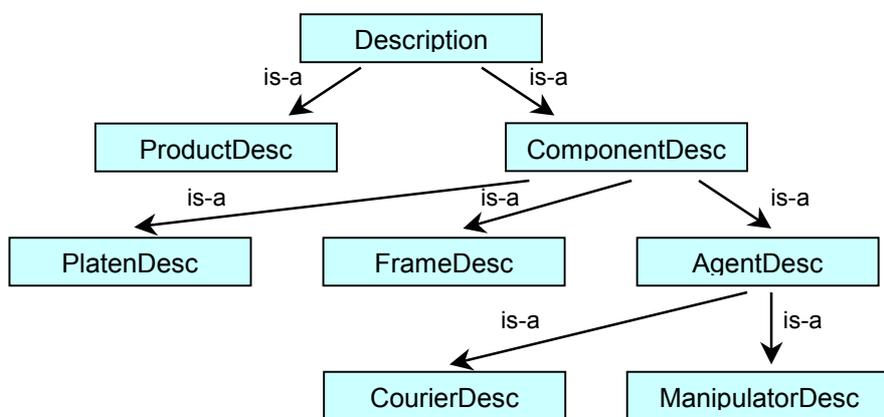
*Figure 6: Class diagram for factory descriptions*
