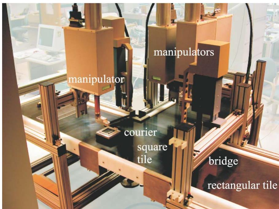
*Figure 1:* T-shaped Minifactory at MSL
