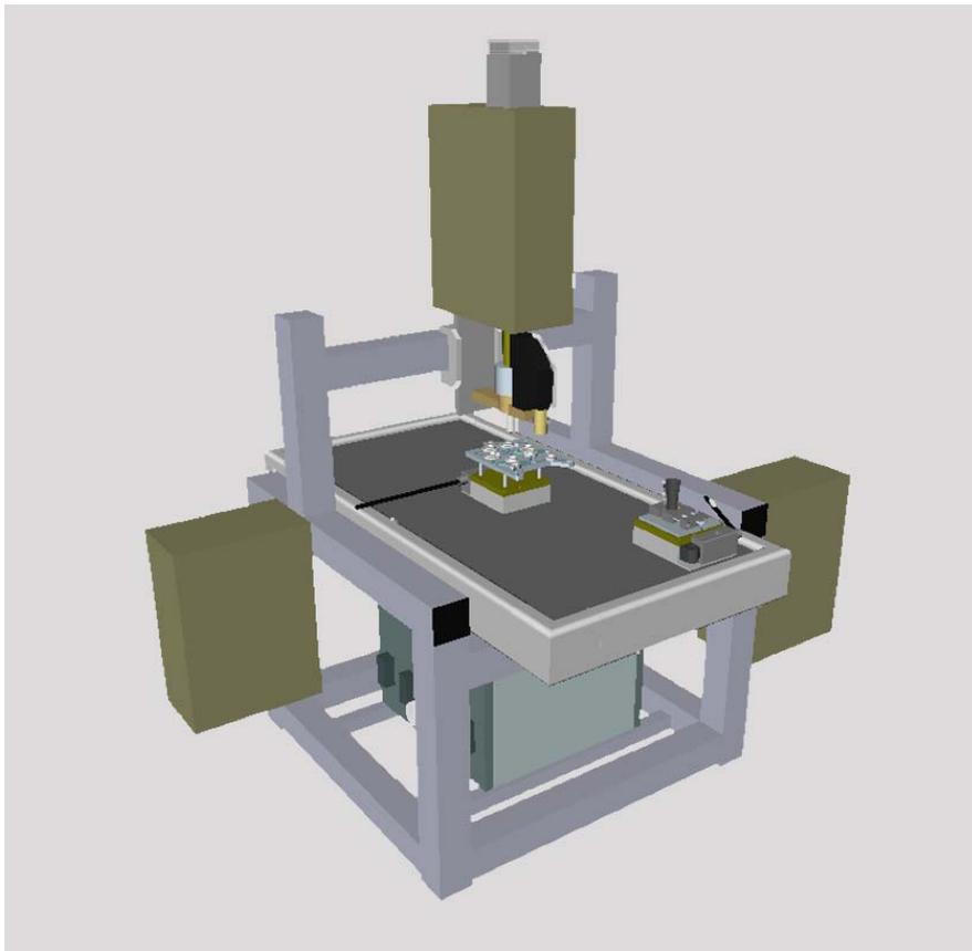
*Figure 14: Set up of the OSTI Minifactory*
